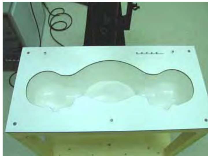
Fig. 5.3 Top view of twin phantom
