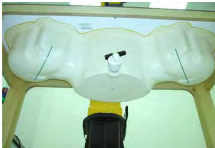
Fig. 5.4 Bottom view of twin phantom
