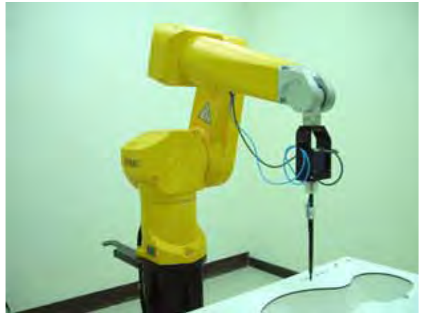
Fig. 5.2 Probe setup on robot
