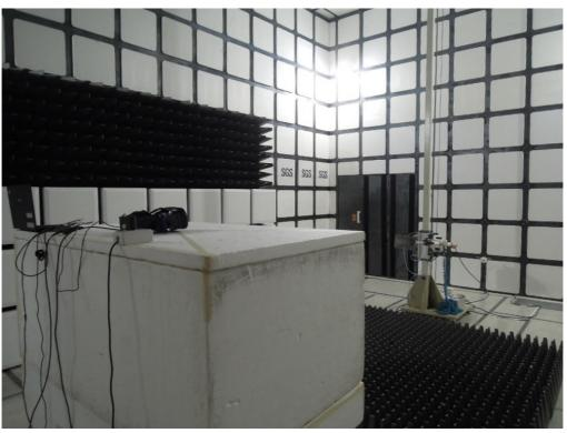
Radiated Emission Set up Photos (Above 1GHz)
