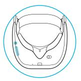
Press the Volume buttons on the bottom left side of the headset or the right side of the controller to adjust the volume.
