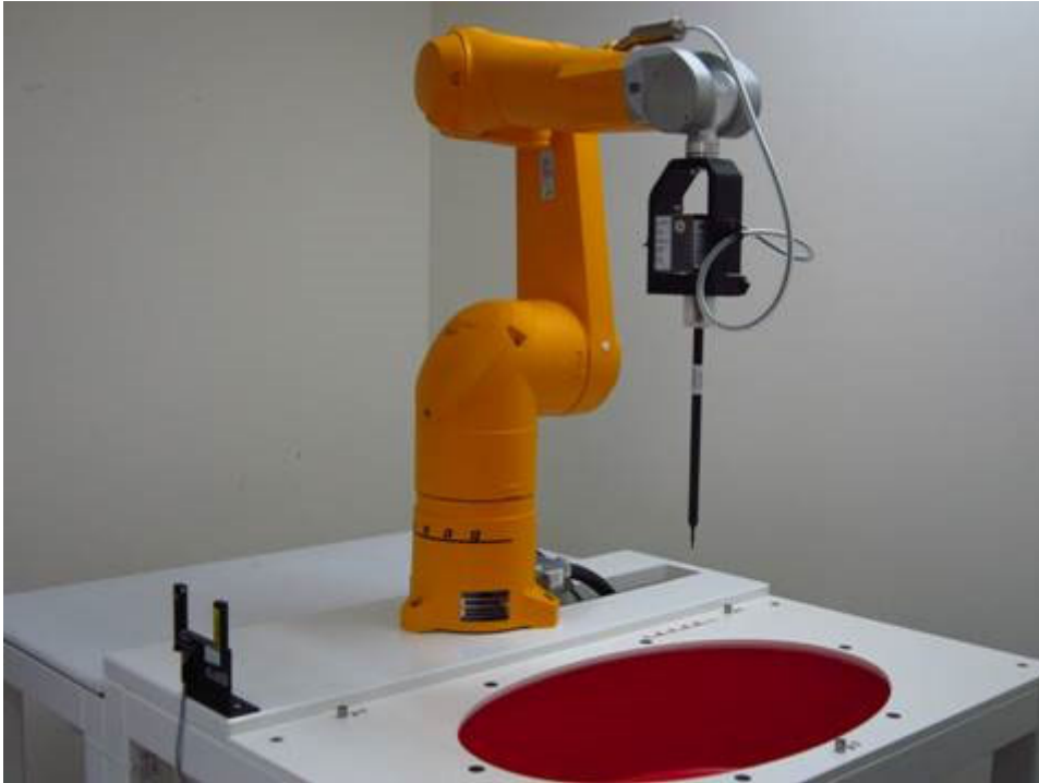
Fig.1 Photograph of the SAR measurement system
