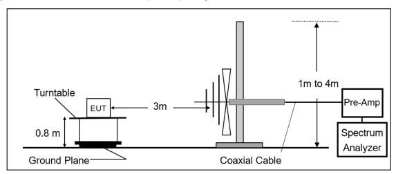
(C) Radiated Emission Test Set-Up, Frequency Above 1GHz.
