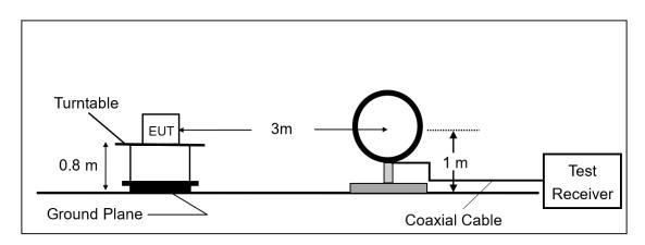
(B) Radiated Emission Test Set-Up, Frequency From 30MHz to 1000MHz.
