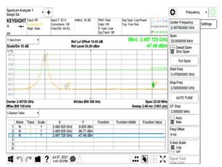
Spurious Emission\_BLE 1M\_LowCH00-2402MHz
