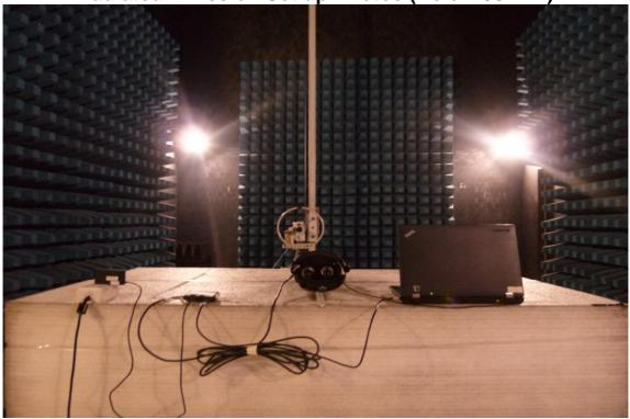
Radiated Emission Set up Photos (Below 1GHz)
