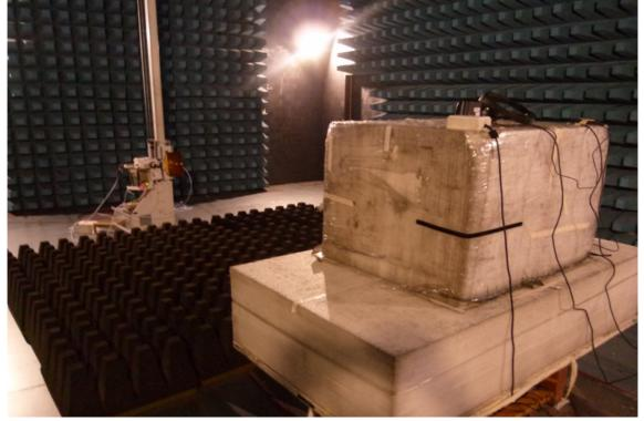
Radiated Emission Set up Photos (Front View)
