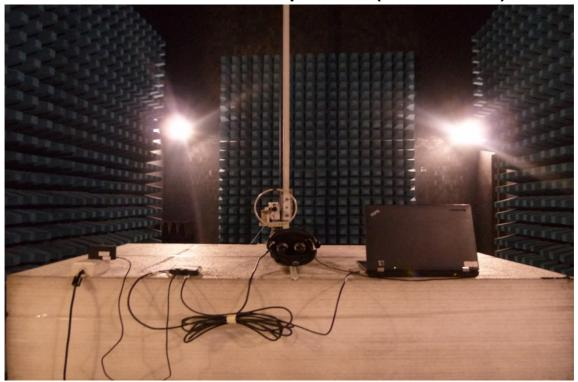
Radiated Emission Set up Photos (Below 1GHz)
