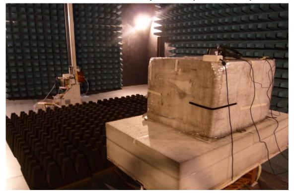
Radiated Emission Set up Photos (Front View)
