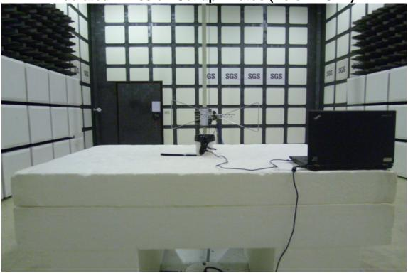
Radiated Emission Set up Photos (Above 1GHz)
