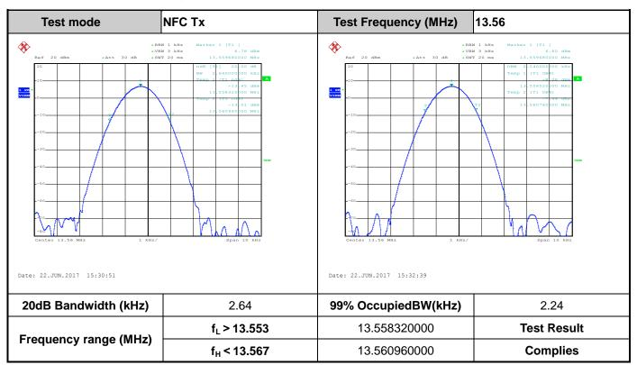
B1. Test Result of 20dB Spectrum Bandwidth
