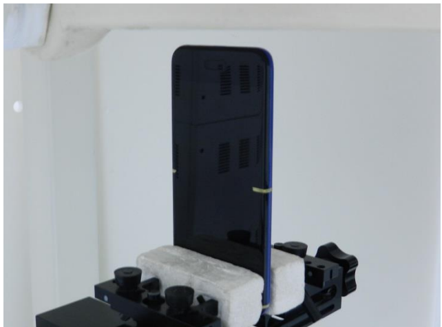
Bottom Side, Test Separation 10 mm
