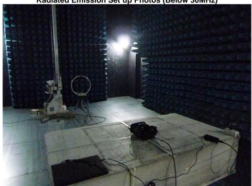
Radiated Emission Set up Photos (Below 1GHz)
