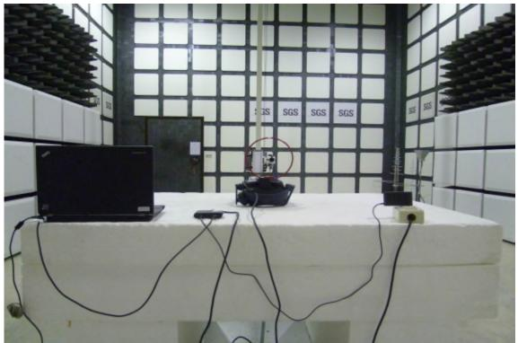
Radiated Emission Set up Photos (Below 1GHz)
