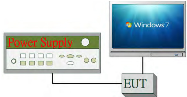
Fig 2-2 Conducted (Antenna Port) Emission Configuration
