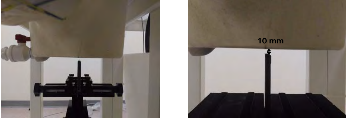
Fig.12 EUT Top side to flat phantom
