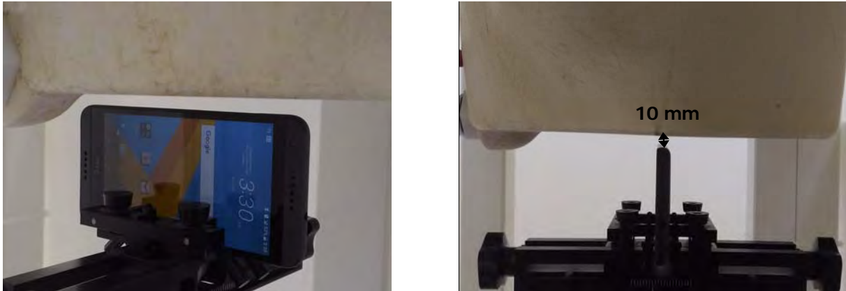
Fig.13 EUT Left side to flat phantom
