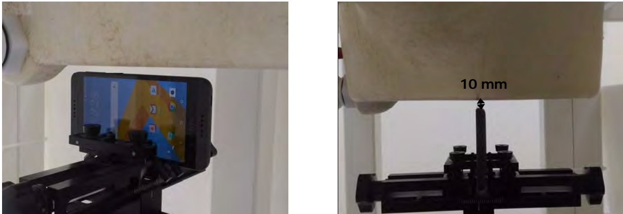
Fig.14 EUT Right side to flat phantom
