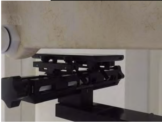
Fig.9 EUT Front side to flat phantom
