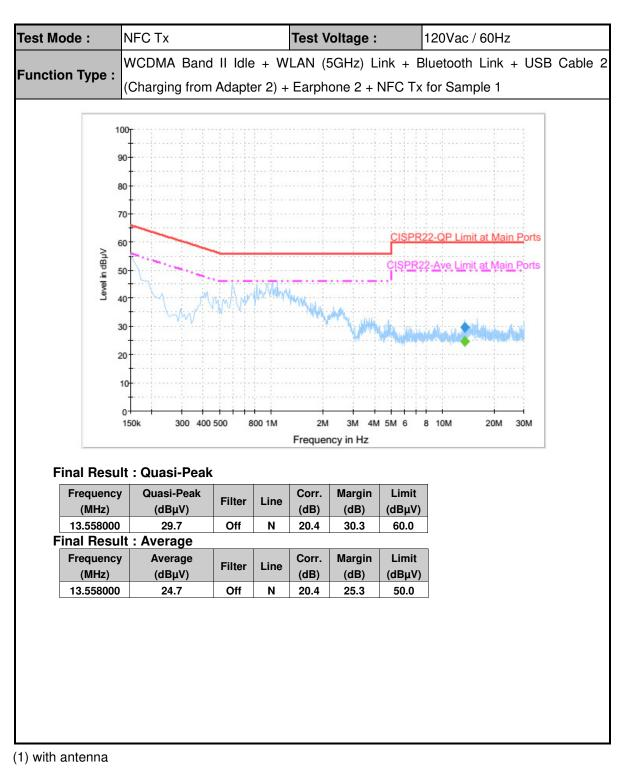
Remark: 13.558MHz is the NFC RF fundamental signal.
