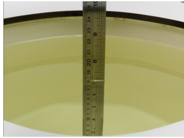
Fig 10.2 Photo of Liquid Height for Body SAR
