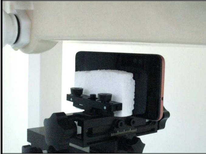
Left Side of EUT with 1.0 cm Gap
