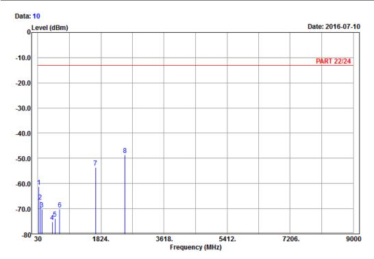
Site : 966 chamber 1 Condition: PART 22/24 Vertical Remark : GSM 850\_Link\_CH189
