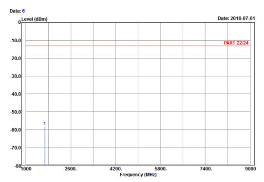
Site : 966 chamber 1 Condition: PART 22/24 Vertical Remark : EDGE 850\_Link\_CH189
