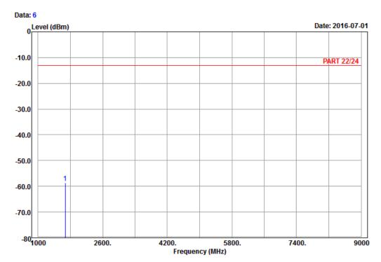
Site : 966 chamber 1 Condition: PART 22/24 Vertical Remark : Band V\_Link\_CH4182
