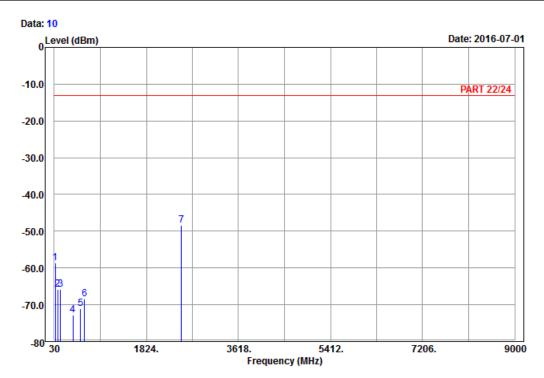
Site : 966 chamber 1 Condition: PART 22/24 Vertical Remark : GSM 850\_Link\_CH189 Tested by: Charles Hsiao
