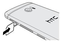
3. Push the tip all the way into the hole until the tray ejects, and then pull the tray out.
