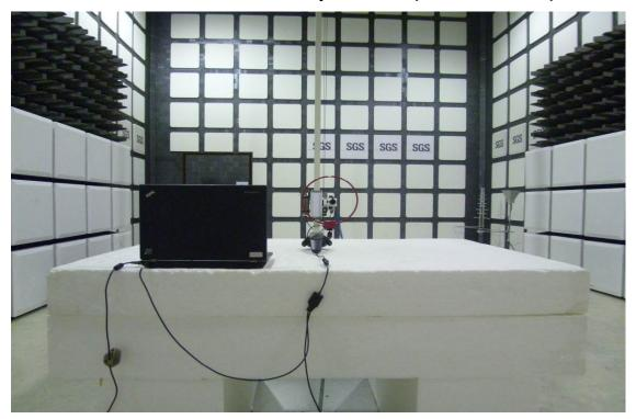
Radiated Emission Set up Photos (Below 1GHz)
