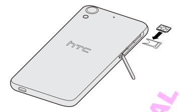
5. Make sure the tray is facing up. Reinsert the tray into the slot.
