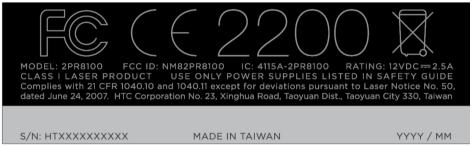
This product contains Class 3B laser, which can produce hazardous level of Class 3B and 4 laser radiations. However, the design of this product incorporates optics, a protective housing and scanning safeguard such that there is no access to level of laser radiation above Class 1. Only trained factory service personnel should open the protective housing.
