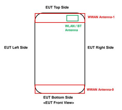
The separation distance for antenna to edge:
