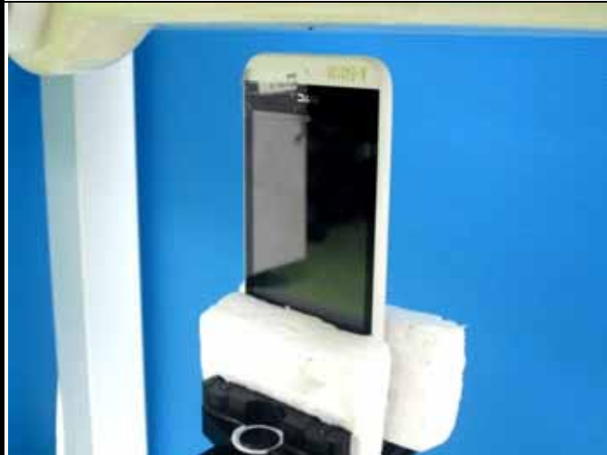
Bottom Side of EUT with 1.0 cm Gap
