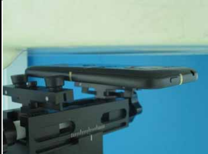
Rear Face of EUT with 1.0 cm Gap
