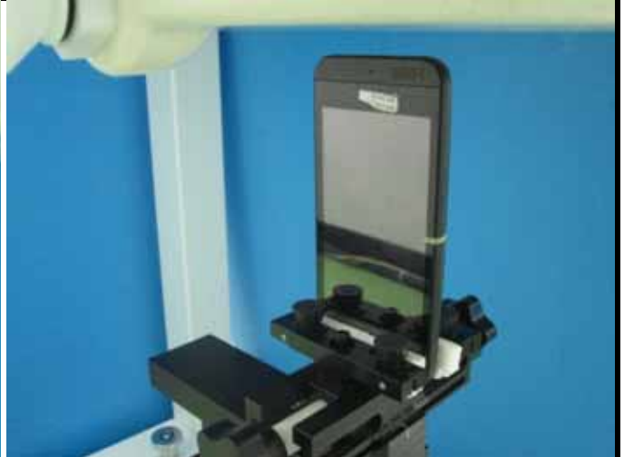
Bottom Side of EUT with 1.0 cm Gap
