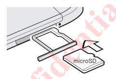
5. Insert the microSD card tray back into the slot.
