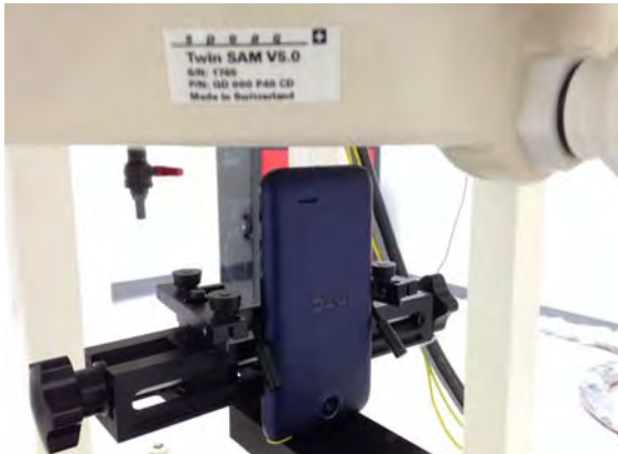
Fig.12 EUT bottom to flat phantom
