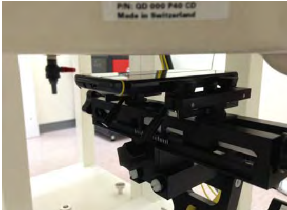
Fig.7 EUT front to flat phantom
