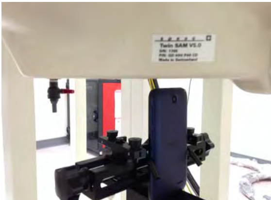
Fig.11 EUT top to flat phantom
