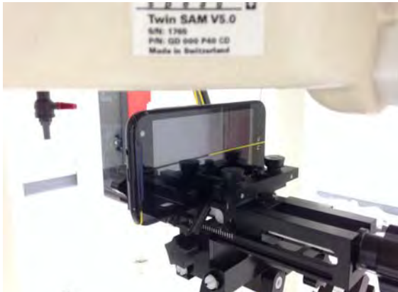
Fig.13 EUT right to flat phantom
