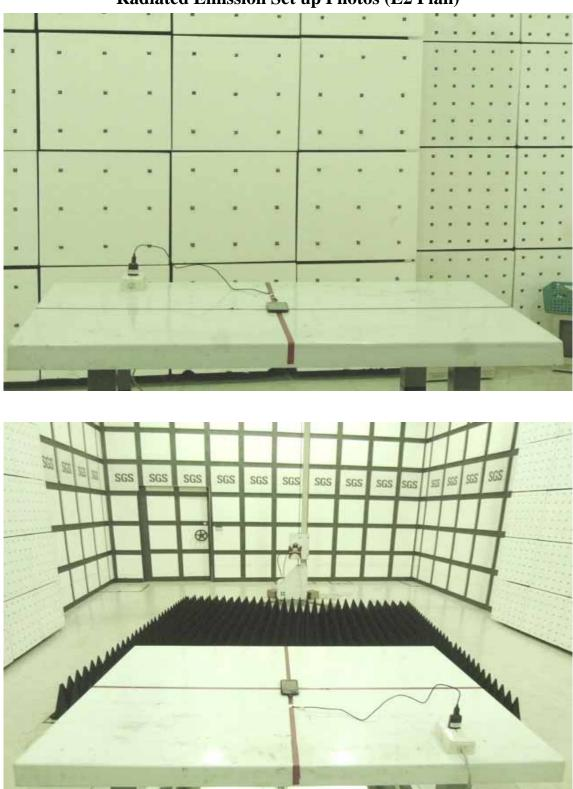
**Radiated Emission Set up Photos (E2 Plan)**
