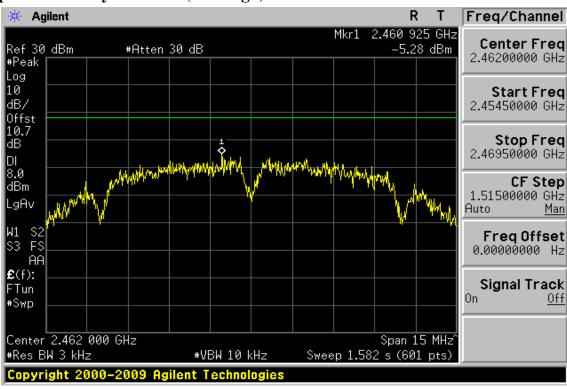
802.11g **Power Spectral Density Test Plot (CH-Low)**
