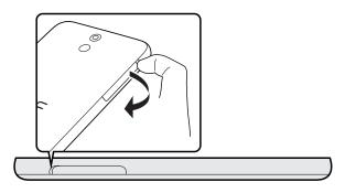
2. With HTC Desire 610 facing down, make sure that the card's gold contacts are facing up and its cut-off corner facing in.
