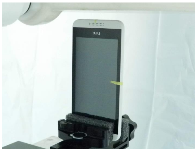
Bottom Side, Test Separation 1 cm
