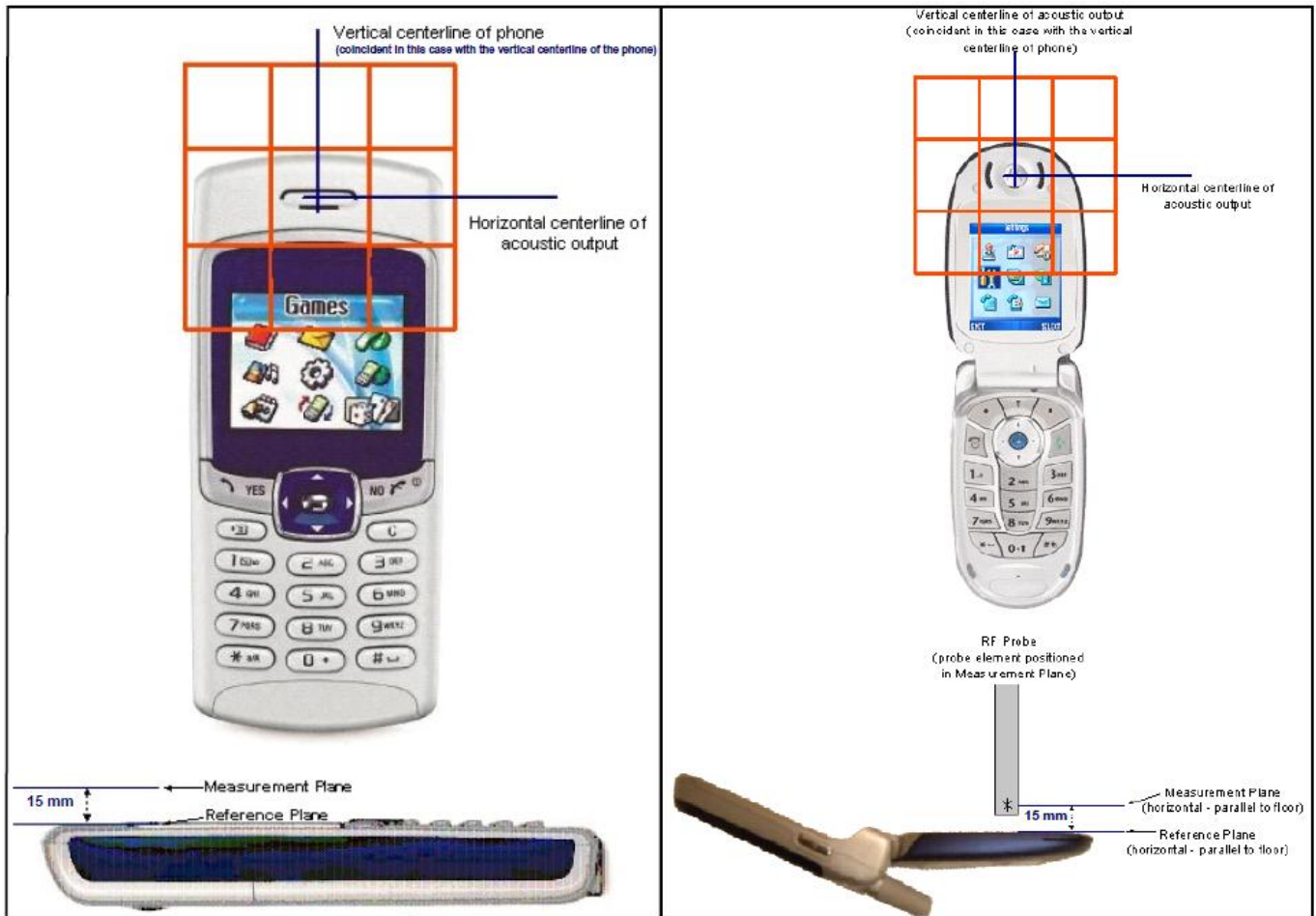
Fig-3.4 EUT Reference and Plane
