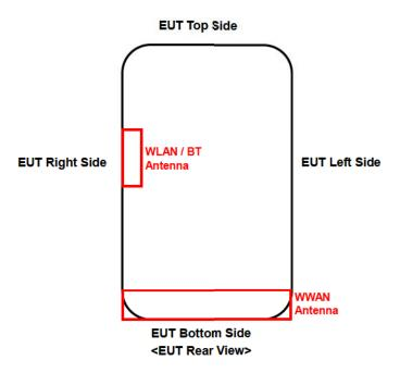
The separation distance for antenna to edge:
