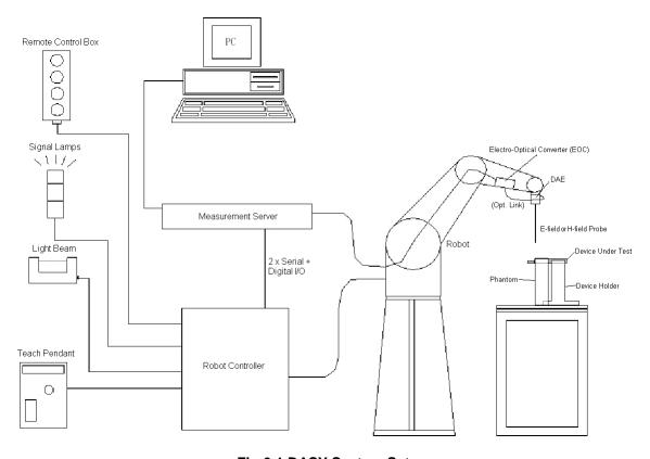
Fig-3.1 DASY System Setup
