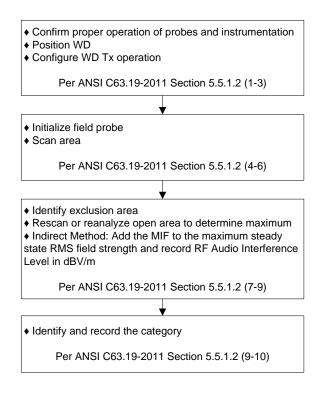
Fig-3.6 WD Near-Field Emission Test Flowchart
