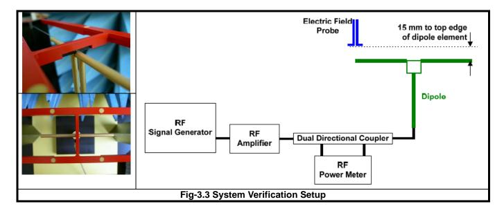
The validation dipole is placed beneath the center of arch phantom. The power meter measures the forward power at the location of the system check dipole connector. The signal generator is adjusted for the desired forward power, 100 mW (20 dBm) at the dipole connector and the RF power meter is read at that level. After connecting the cable to the dipole, the signal generator is readjusted for the same reading at RF power meter.
