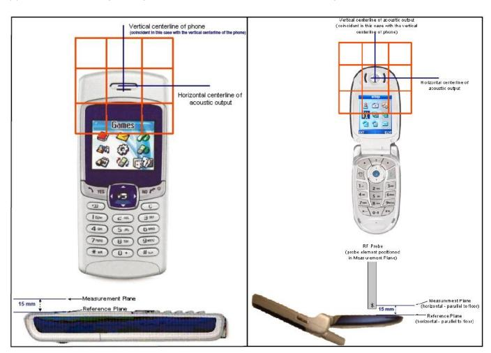
Fig-3.4 EUT Reference and Plane
