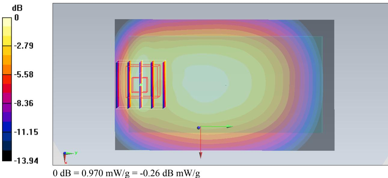
**#42\_GSM850\_DTM Multi-slot class 11\_Back\_1cm\_Ch128****DUT: 370213**
