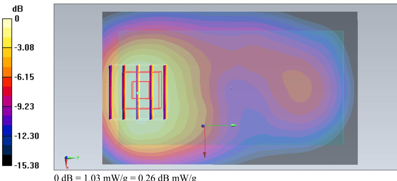
**#51\_GSM1900\_GPRS (4 Tx slots)\_Back\_1cm\_Ch661****DUT: 370213**
