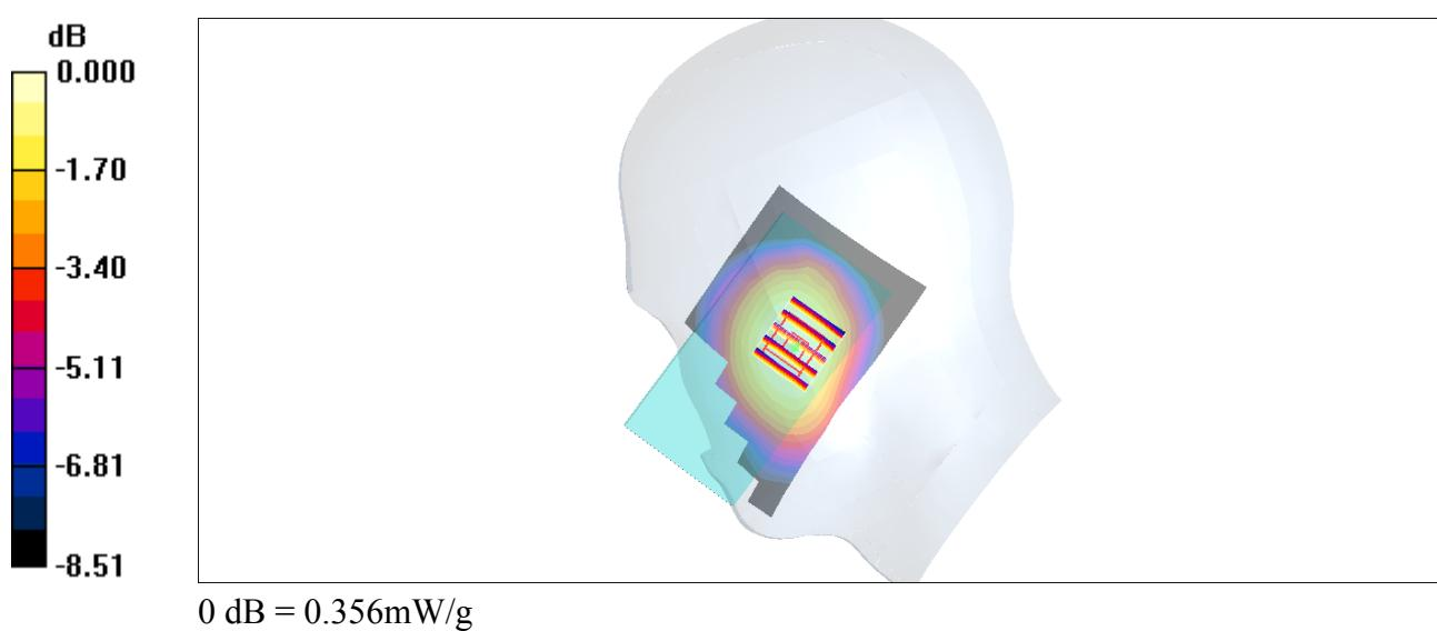
**#59\_GSM850\_DTM Multi-slot class 11\_Left Cheek\_Ch251****DUT: 370213**
