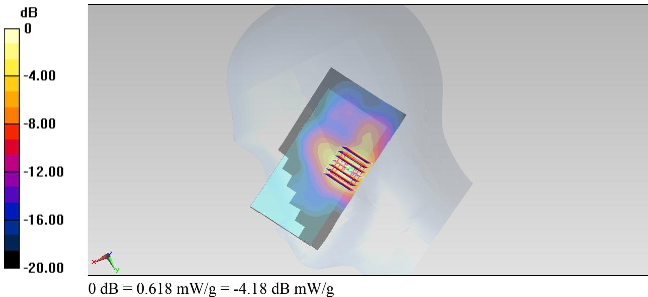
**#80\_WLAN2.4GHz\_802.11b 1Mbps\_Right Tilted\_Ch6****DUT: 370213**
