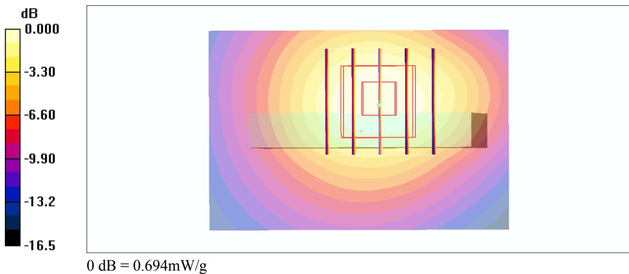
**#07\_GSM1900\_DTM Multi-slot class 11\_Front\_1cm\_Ch512****DUT: 370213**
