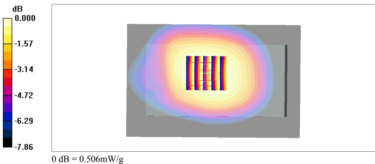
**#33\_GSM850\_GPRS (4 Tx slots)\_Back\_1cm\_Ch251****DUT: 370213**
