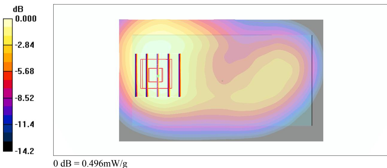
**#02\_GSM1900\_GPRS (4 Tx slots)\_Back\_1cm\_Ch512****DUT: 370213**
