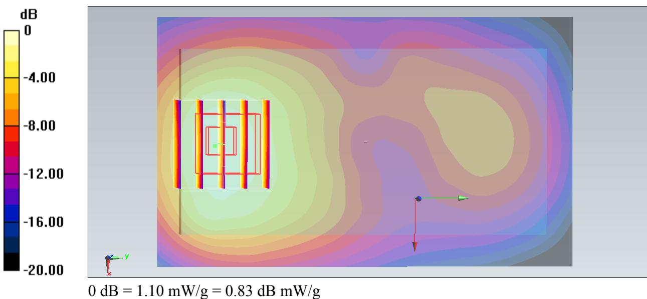
**#52\_GSM1900\_GPRS (4 Tx slots)\_Back\_1cm\_Ch810****DUT: 370213**
