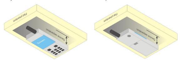
Fig 8.4 Illustration for Body Worn Position
