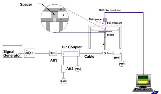
Fig 7.1 System Setup for System Evaluation
