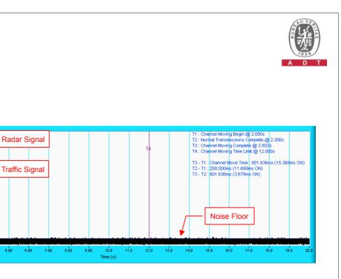
NOTE: T1 denotes the start of Channel Move Time upon the end of the last Radar burst. T2 denotes the data transmission time of 200ms from T1. T3 denotes the end of Channel Move Time.T4 denotes the 10 second from T1 to observe the aggregate duration of transmissions.
