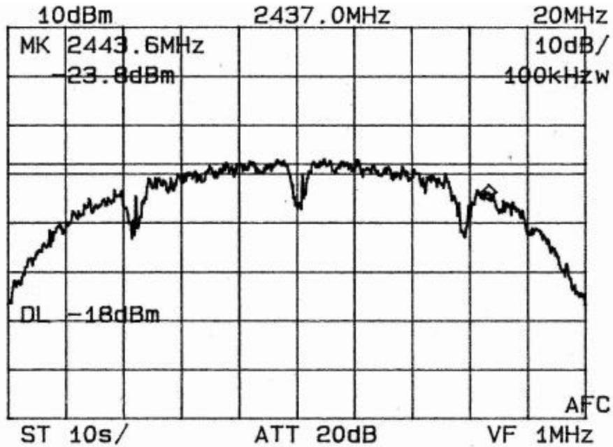
**4.2.3 6 dB Bandwidth Emissions (100 kHz Res. BW) High Channel Bandwidth Plot:**
