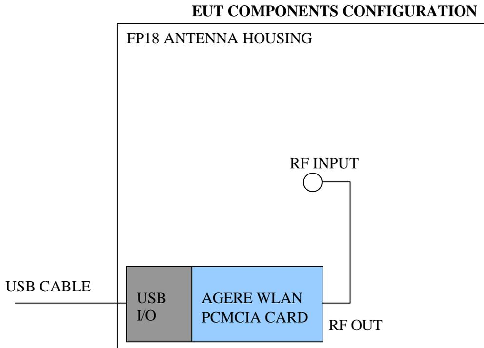
The USB interface and WLAN card are contained inside the antenna housing.
