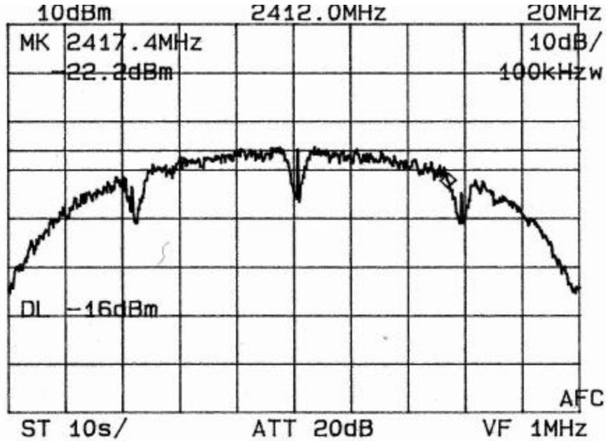
**4.2.2 6 dB Bandwidth Emissions (100 kHz Res. BW) Mid Channel Bandwidth Plot:**
