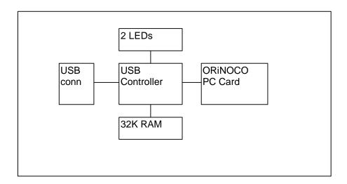
The USB controller is the core of the product. This chip interfaces between the USB bus and the PC Card interface. The chip consists of an 8051 CPU and 8K RAM. The program code is downloaded from the USB host into the device. For future software updates, additional RAM is provided [32KByte].
