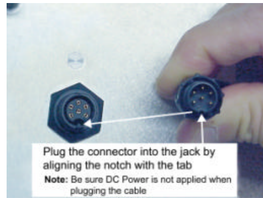
Figure 6 – Plugging the Round Connector
