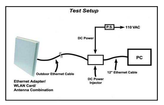
The LAN interface and WLAN card are contained inside the antenna housing.
