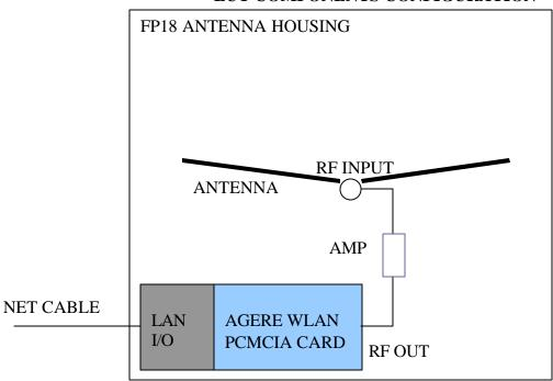
The LAN interface and WLAN card are contained inside the antenna housing.
