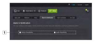
Camera has ability to send event notifications when motion or audio is detected.
