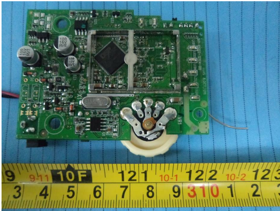
EUT – Main Board shielding off Top View
