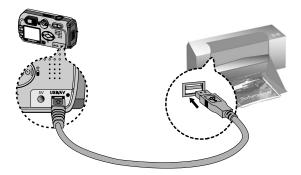
If you selected [COMPUTER] in Step 5, when you connect the camera to your printer, the Mode dial lamp(Green) will illuminate and the connection will not be established. In this case, disconnect the USB cable, and then follow the procedure from Step 2 and onward.
