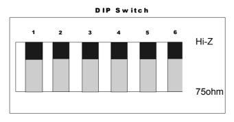
To configure the function of the six coaxial cable ports at the rear of Webthru SWC 306.
