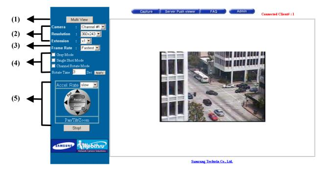
At default viewer, a user may configure image transmission method and control integrated PTZ mechanism of a CCTV camera. The PTZ control panel is activated in some seconds depending on network speed.
