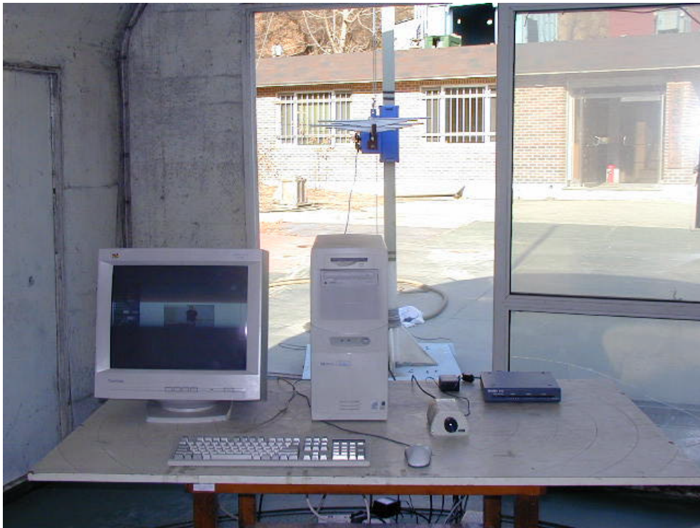
RADIATED EMISSION SETUP PHOTOGRAPH - FRONT VIEW ( 300- 1000 MHz )
