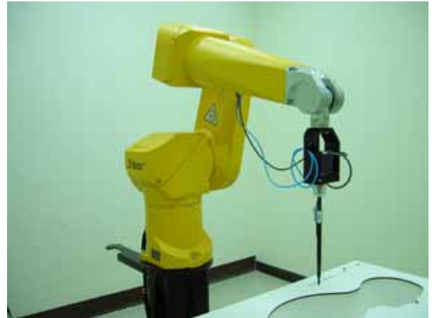
Fig. 5.2 Probe setup on robot
