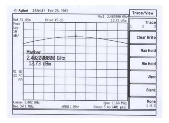
At the 2402Mhz , The measured power is 12.73 dbm +0.4db(cable loss)
