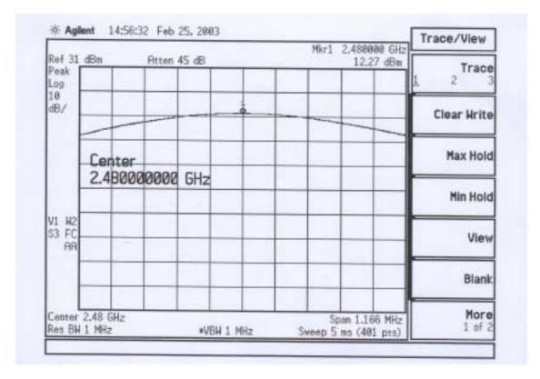
At the 2480 Mhz, The measured power is 12.27 dBm + 0.4 db = 12.67 dbm
