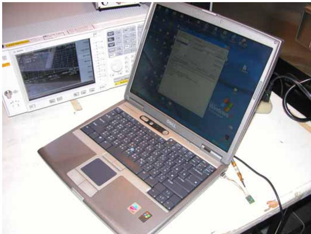
**POWERLINE CONDUCTED EMISSIONS MEASUREMENT SETUP**
