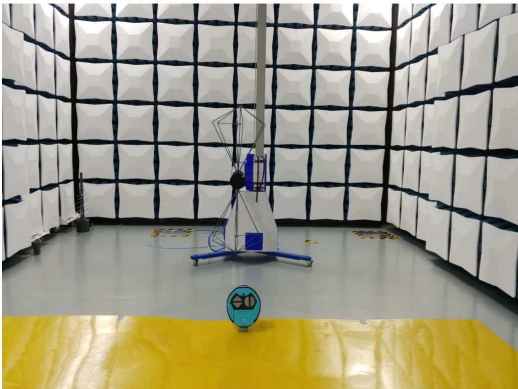
Set-up for Radiated Emission (30-200MHz)
